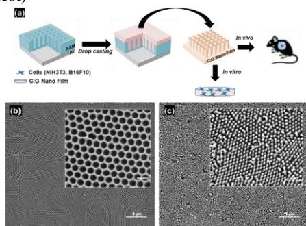
Figure 1. Schematic representation of study (a). SEM images of AAMs (b) and nano- films (c).
