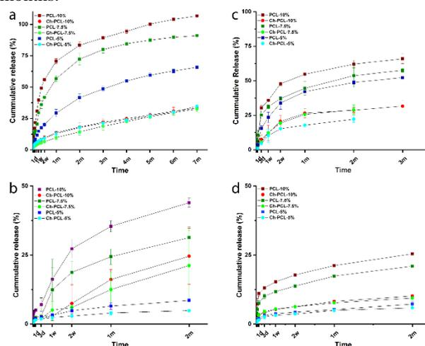
**Figure 1.** Release profile of (a) BSA (b) bevacizumab from 1.645 mm inner diameter capsule; (c) BSA (d) bevacizumab from 260  $\mu$ m inner diameter capsule
