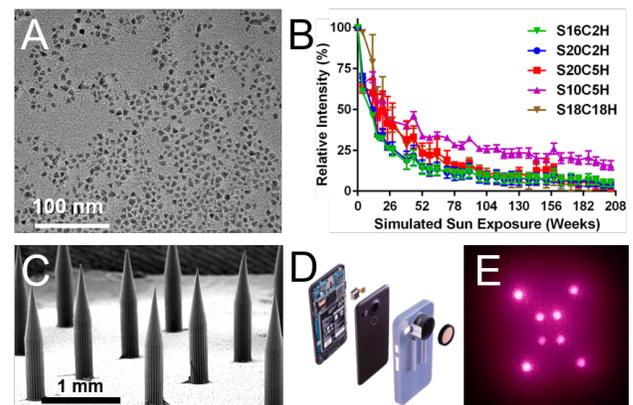
Figure 1. Near-infrared quantum dot synthesis, evaluation, and application. (A) Transmission electron microscopy image of copper-based quantum dots. (B) photostability of quantum dots under simulated sun exposure through skin. (C) Scanning electron microscopy image of microneedles. (D) Adapted smartphone with internal near-infrared filter removed and long-pass filters added. (E) “X” pattern detected using the adapted smartphone following microneedle administration to rats.
